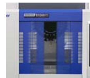
Automatic door (motor-driven)
